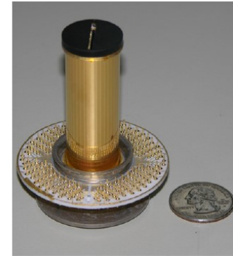
Texas Instrument 180—photoconductive MCT element Common Module FPA mounted on a dewar stem (M.A. Kinch, "Fifty years of HgCdTe at Texas Instruments and beyond," Proc. SPIE 7298 (2009))
