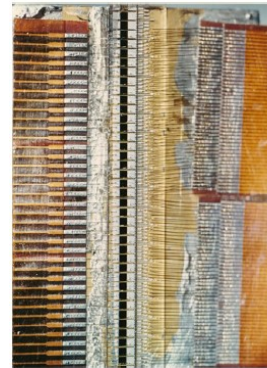
Texas Instrument 180—photoconductive MCT element Common Module FPA mounted on a dewar stem (M.A. Kinch, "Fifty years of HgCdTe at Texas Instruments and beyond," Proc. SPIE 7298 (2009))
