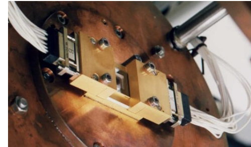
HRIS 128x140 pixels SWIR MCT array built by GMIRL (formerly Mullard Lab and Philips PICS now Leonardo UK) and tested in Matra Marconi Space detection
