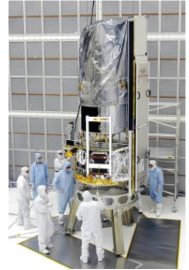
Spitzer IR observatory launched in 2003, notably using 256x256 InSb and Si:As BIB arrays (IRAC) as well as 128x128 Si:As and Si:Sb arrays (IRS) ( https://en.wikipedia.org/wiki/Spitzer_Space_Telescope )
