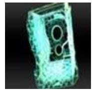
This updated software now features an X-Ray Mode which is capable of examining raw scan data for potential problem areas before it enters the processing stage. The new X-ray Mode makes raw scan data semi-transparent and deletes all the noise around a scanned object, showing users the data that they want to see. This new function makes raw scan data semi-transparent while deleting the noise around a scanned object, to show users the desired data.
