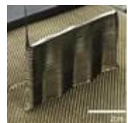
Schroers and colleagues simplifies the additive manufacturing of metallic components by exploiting the unique-amongst-metals softening behavior of BMGs. Due to the similarity between FFF of thermoplastics and BMGs, this method may leverage the technology infrastructure built by the thermoplastic
