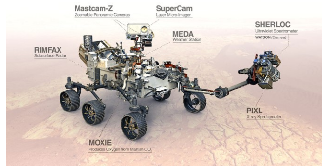
Fig. 1. The Mars 2020 Perseverance Rover, with the seven scientific instruments labeled. NASA/JPL-Caltech
