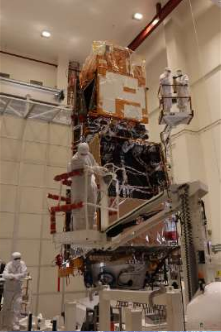
IASI PFM integration on METOP-SG A1 platform
