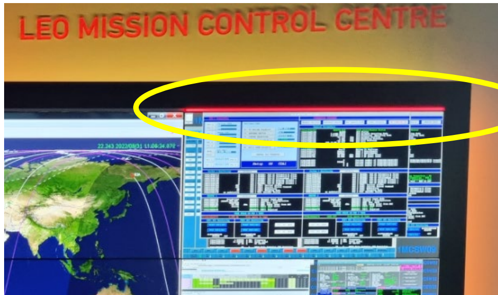
(Fig.11) LED strap indicating an alarm on video wall monitor
