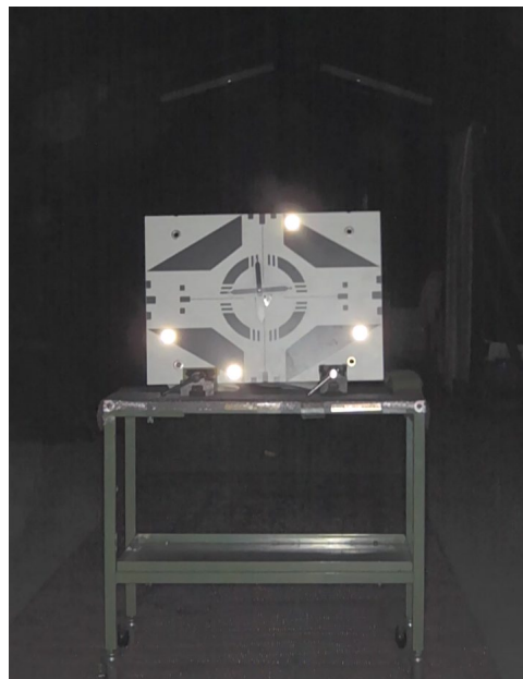
Fig.11 Dark place camera imaging test with LED light using CDT mock-up
